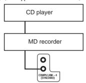
TEXT COMPU LINK jacks: Use the cables with the stereo mini-plugs (not supplied with this receiver).
